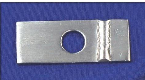
Welded coupons can be prepared with or without the use of filler metal. The autogenous weld is prepared without the use of filler metal. This type of weld is the most economical method. Autogenous welds are commonly used to evaluate corrosion rates of welded materials and the usage of these materials in corrosive environments. An autogenous weld is produced by GTAW and can be used to test material weldability and gas shield usage, and to set welding parameters.
