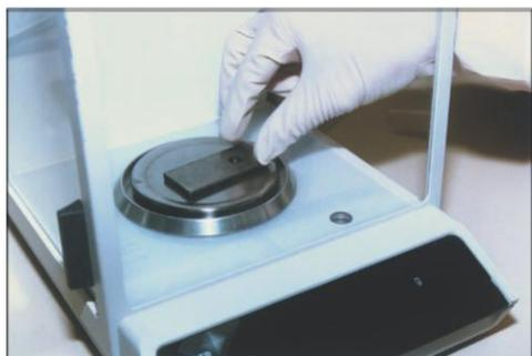
Metal Samples offers post exposure coupon analysis. Our trained technicians will perform weight loss analysis and determine mils per year (MPY) corrosion rates of your exposed test samples. We are in adherence to ASTM-G1 specifications for cleaning and analyzing coupons.
